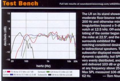
The LR on its stand showed a moderate floor-bounce notch at 200 Hz and otherwise minor irregularities beyond a 5-dB notch at 12.5 kHz. Off-axis lobing of the center began with the mike at 22.5°, and the surrounds exhibited the notching considered desirable in bidirectional speakers. The subwoofer displayed moderate dynamic capability, but SPL was very evenly distributed, and the unit delivered 103 dB or greater at any frequency above 25 Hz. Max SPL measured 106 dB at 62 Hz. - Tom Nousaine
